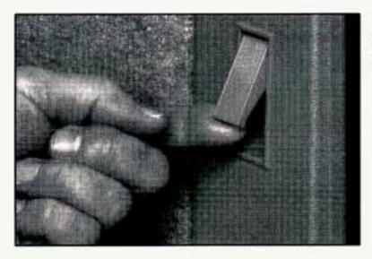
Lift up on the latch and pull the jack cover off.
